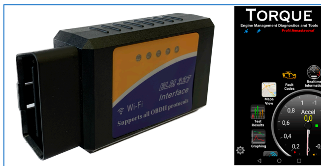
Figure 5. ELM 327 Diagnostic Tool and Torque Pro Mobile App [author].
