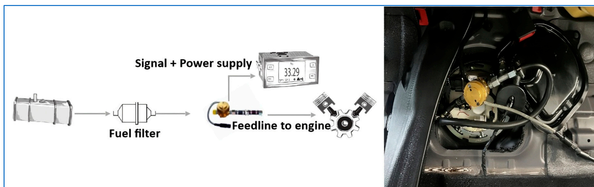
Figure 6. AIC 1204 flow meter and its connection method [21].
