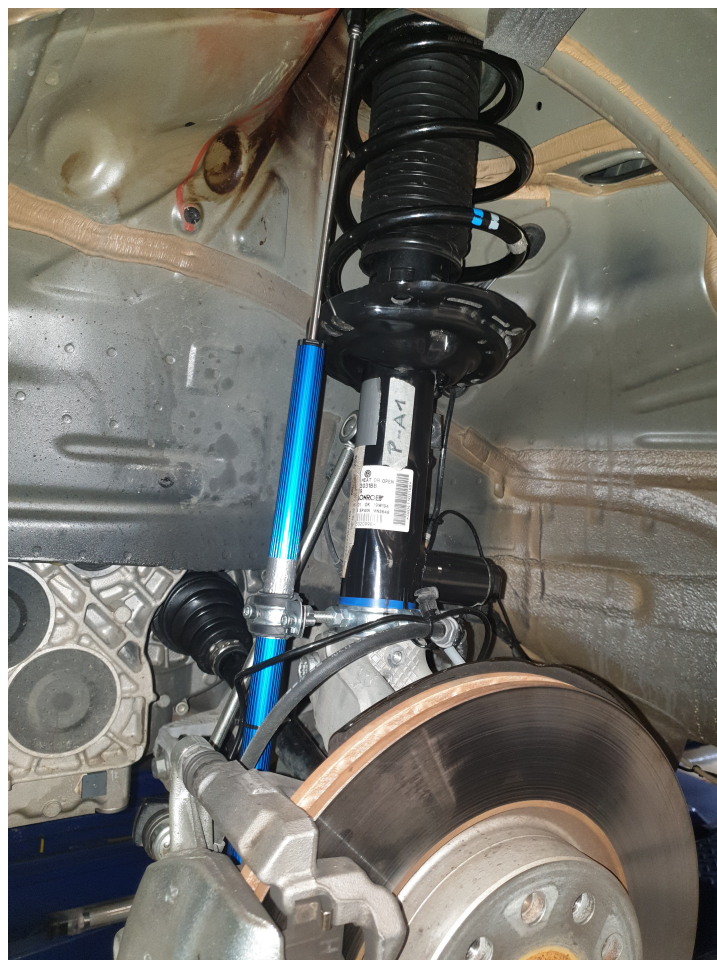
Figure 4. Shock absorber stroke measurement during driving tests.
