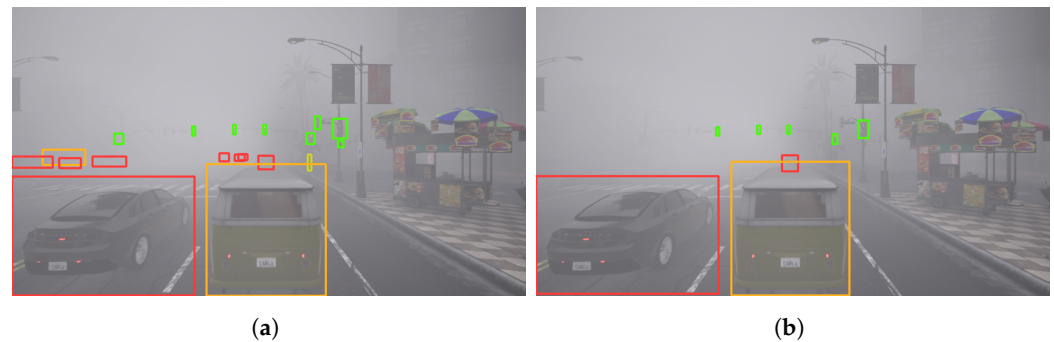
Figure 3. We tested our object detection model in heavy fog conditions (fog density 100%) using a model that was trained with labels for all objects up to 200 m. The model trained with data under fog density 100% outperformed the model trained on clear data in detecting objects at long distances. As shown in (a), on the left, the fog-trained model successfully detected distant objects, while the clear-data model struggled to do so, as evident in (b) on the right. This difference in performance primarily increases the recall of the model. The red box describes the cars, the orange box describes the vans, and the green box describes the traffic lights.
