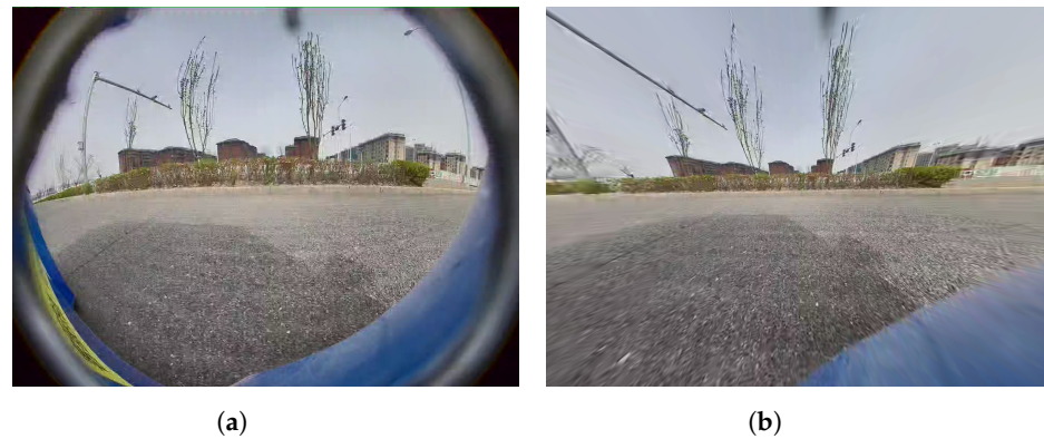
Figure 4. Fisheye camera undistortion test visualization. (a) Raw fisheye camera image. (b) Rectified fisheye camera image using Kannala–Brandt model.
