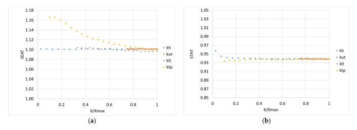
**Figure 12.** (a) SEAT and (b) STHT values versus the stiffness coefficient values of the driver's body parts for the periodic excitation.
