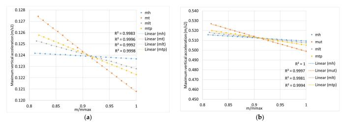
**Figure 4.** Maximum value of driver's head acceleration versus the value of mass for the **(a)** speed bump and **(b)** pothole excitation.
