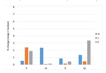
**Figure 15.** Change in RMS acceleration of the driver's head over the values of the lumped parameters for the periodic excitation.
