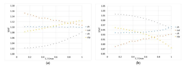
**Figure 13.** (a) SEAT and (b) STHT values versus the damping coefficient values of the driver's body parts for the periodic excitation.
