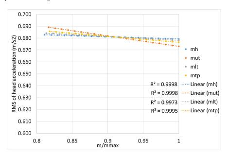
Figure 5. RMS value of driver's head acceleration versus the value of mass for the periodic excitation.
