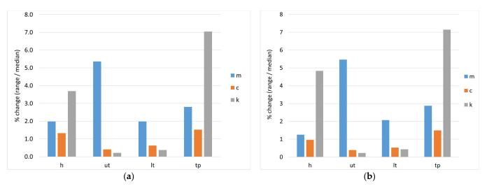
**Figure 14.** Change in maximum acceleration of the driver's head over the values of the lumped parameters for the (a) speed bump and the (b) pothole excitation.
