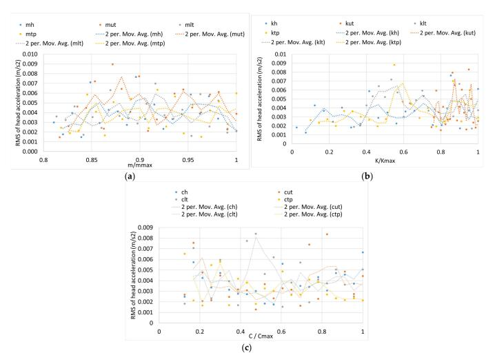
**Figure 10.** RMS value of the driver's head acceleration versus the value of **(a)** mass, **(b)** stiffness and **(c)** damping coefficients for the Grade E road profile.
