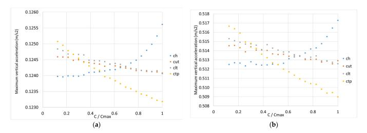
**Figure 8.** Maximum value of driver's head acceleration versus the value of the damping coefficient for the (a) speed bump and (b) pothole excitation.
