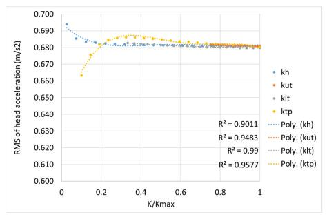
**Figure 7.** RMS value of driver's head acceleration versus the value of the stiffness coefficient for the periodic excitation.
