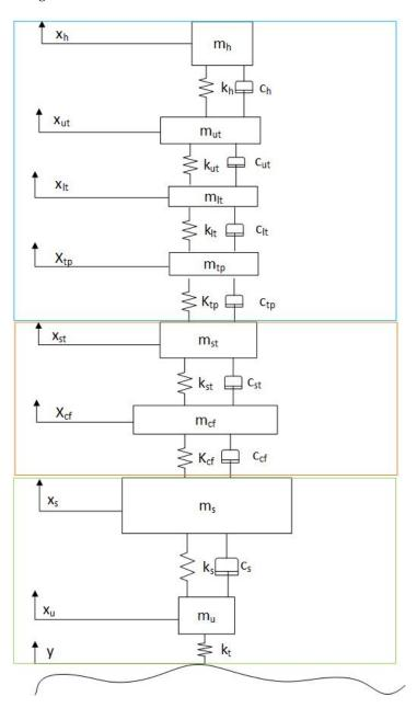
Figure 1. Eight-DOF vehicle–seat–driver lumped-parameter model.
