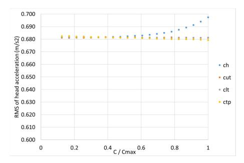
**Figure 9.** RMS value of driver's head acceleration versus the value of the damping coefficient for the periodic excitation.
