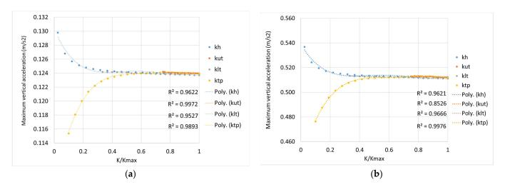
**Figure 6.** Maximum value of driver's head acceleration versus the value of the stiffness coefficient for the (a) speed bump and (b) pothole excitation.
