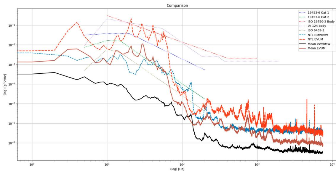
**Figure 10.** Comparison of 95/50 normal tolerance limits for cobble stone and rough cobble stone measurements of VW&BMW vs. EVUM commercial minitruck.
