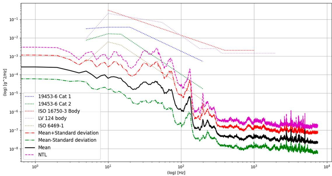
Figure 8. Statistical evaluation of the BMW i3 over all measurement data.
