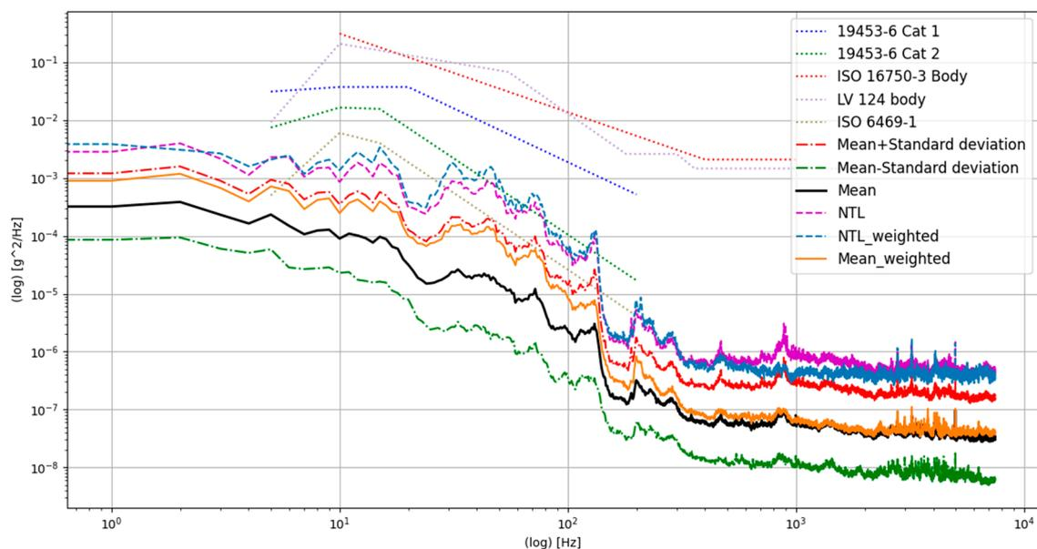
**Figure 11.** Load profile calculated from measurement data.
