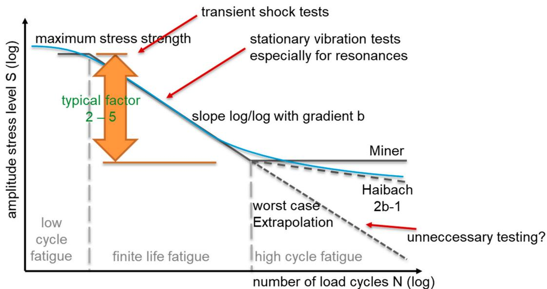
Figure 4. Boundary considerations of fatigue analysis using a typical SN curve.
