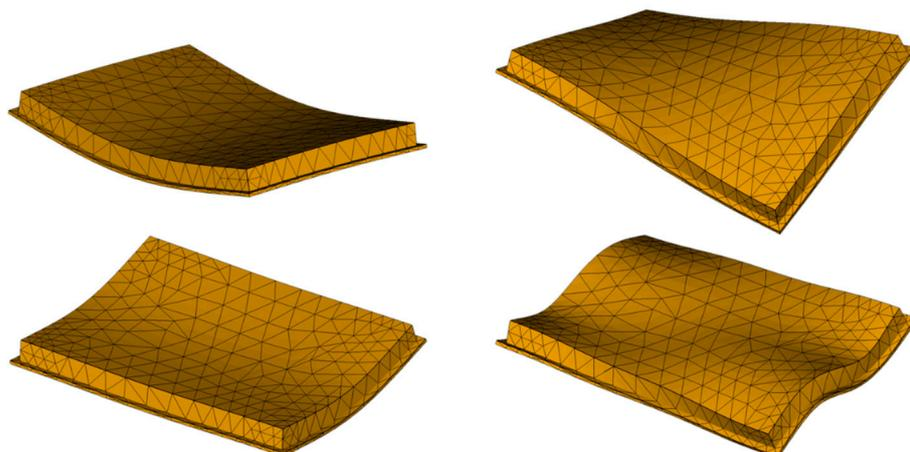
**Figure 3.** First two modes of global bending (**left**), simple mode of global torsion and local corner bending (**right**) for a vehicle floor battery pack, similar to [2].
