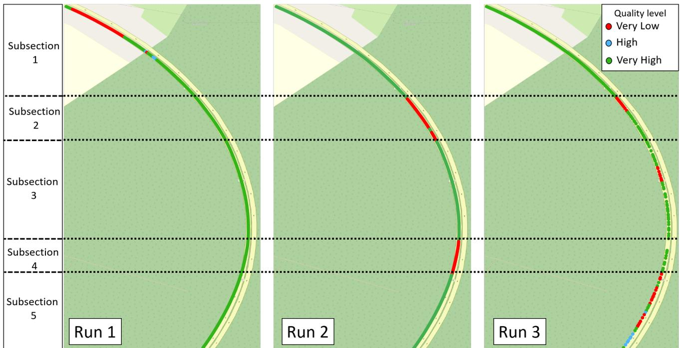
**Figure 12.** Comparison of the Very High rate on road section n°3—Long Curve between the three runs.
