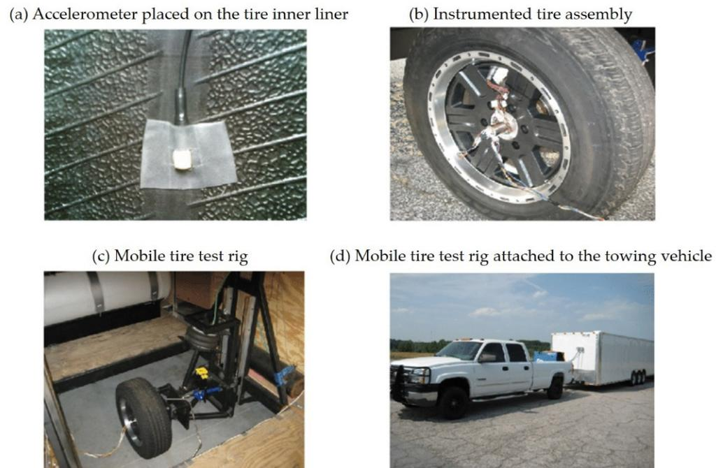
**Figure 11.** Full-scale application of a smart tire system and its components [87].
