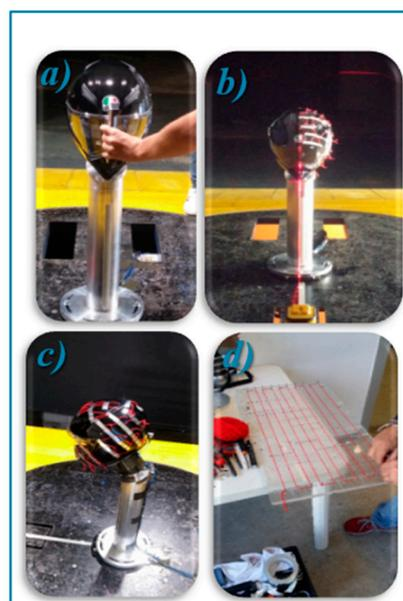
Figure 4. (a) Alignment with respect to the vertical axis; (b) centering; (c,d) application of wool threads.
