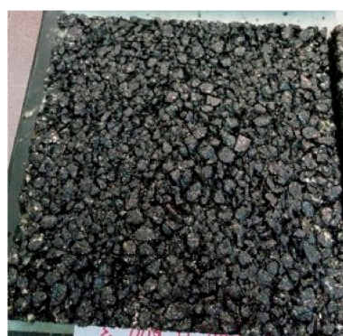
Figure 5. Hot-mix asphalt concrete (HMA) with no modifiers (slabs code: H A ).
