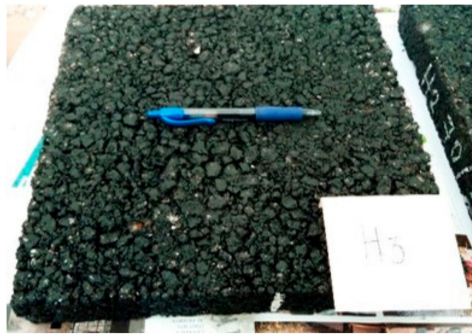
Figure 11. Prepared slabs using RAP material (slabs code: H E ).
