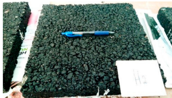
Figure 10. Prepared slabs using RAP material (slabs code: H D ).
