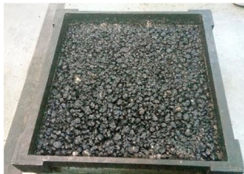
Figure 6. HMA with modifiers for in-situ layering (slabs code: H B ).
