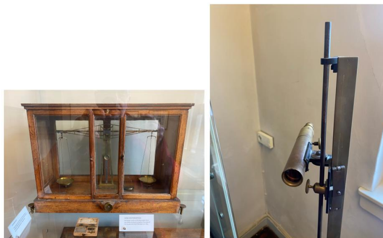
Figure 12. The best balance of Liebig with an accuracy of 0.3 mg and a maximum of 100 g; the telescope used to read the balance.
