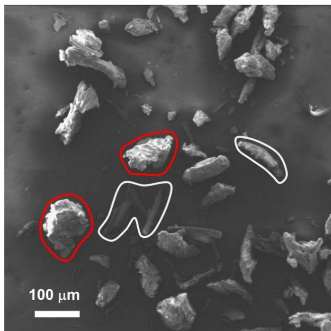
**Figure 2.** SEM image of a physical mixture of cellulose and AC-Air carbon catalyst. Cellulose particles are encircled in red, and AC-Air particles are encircled in white.
