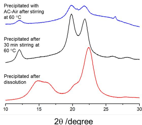
**Figure 5.** X-Ray diffraction patterns of cellulose precipitate after dissolution in H<sub>3</sub>PO<sub>4</sub> under different conditions.
