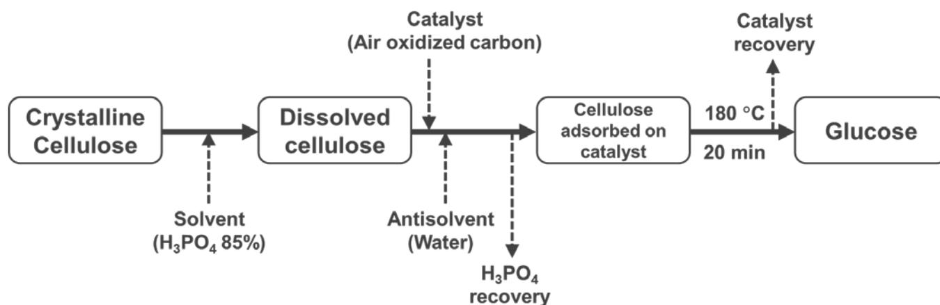
**Figure 3.** Schematic representation of solvent-assisted adsorption process followed by hydrolysis of adsorbed cellulose to obtain glucose.
