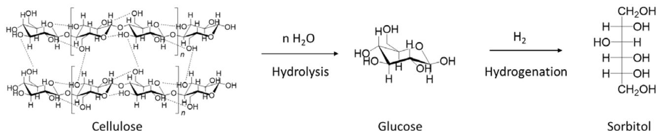
**Figure 1.** Depolymerization of cellulose by hydrolysis to glucose and further hydrogenation to sorbitol.
