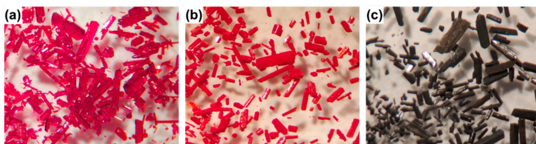
Figure 1. Crystals of (a) \text{Co(L)}\cdot\text{CS}_2 ; (b) \text{Co(L)} , obtained by the desorption of \text{CS}_2 from \text{Co(L)}\cdot\text{CS}_2 ; and (c) \text{Co(NO)}(\text{L}) after the NO gas–solid reaction with \text{Co(L)} .
