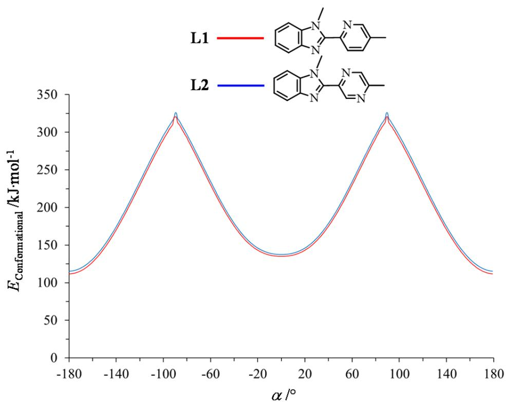
**Figure S10.** Gas-phase energies computed for **L1** and **L2** at the MM2 level using Chem3D as a function of the interplanar angle  $\alpha$  [61].
