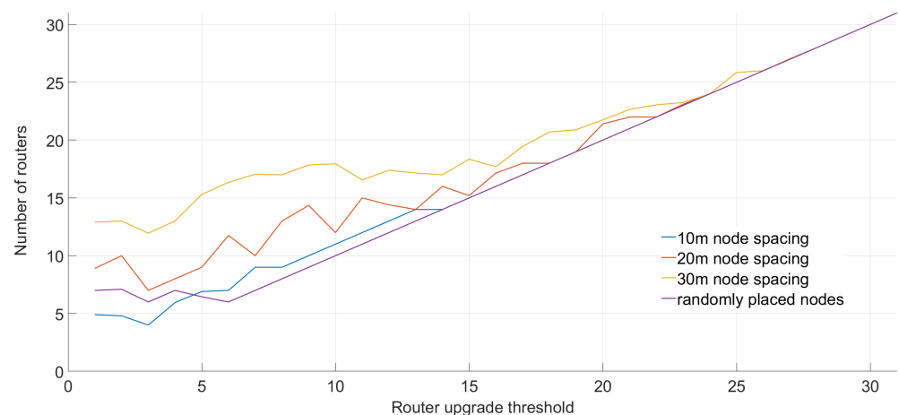
Figure 11. Mean number of routers in different topologies based on 20 simulation runs.
