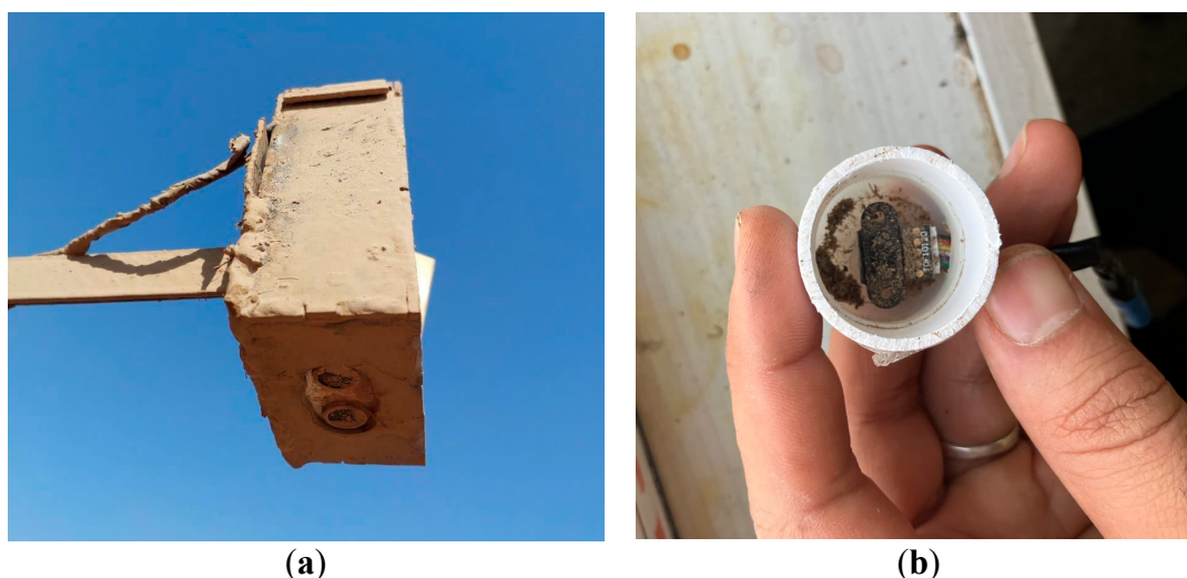
Figure 6. Impact of field conditions on sensor performance: (a) ultrasonic and (b) laser range sensors partially obstructed by dust and displaced soil particles.
