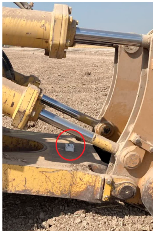
Figure 2. Location of the inclinometer on the subsoiler (outlined in red circle).
