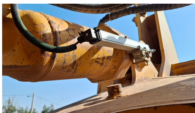
Figure 3. Placement of linear potentiometers in the hydraulic cylinder, used to monitor shank displacement and derive accurate subsoiling depth.
