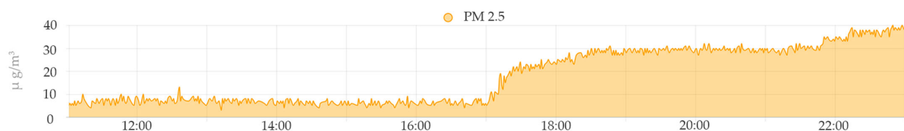
Figure 18. Collected PM 2.5 sample in a space heated by a heat pump (11–17 h) and a wood stove (17–23 h).
