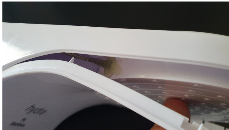
Figure 14. Detail of the installation of the temperature sensor.
