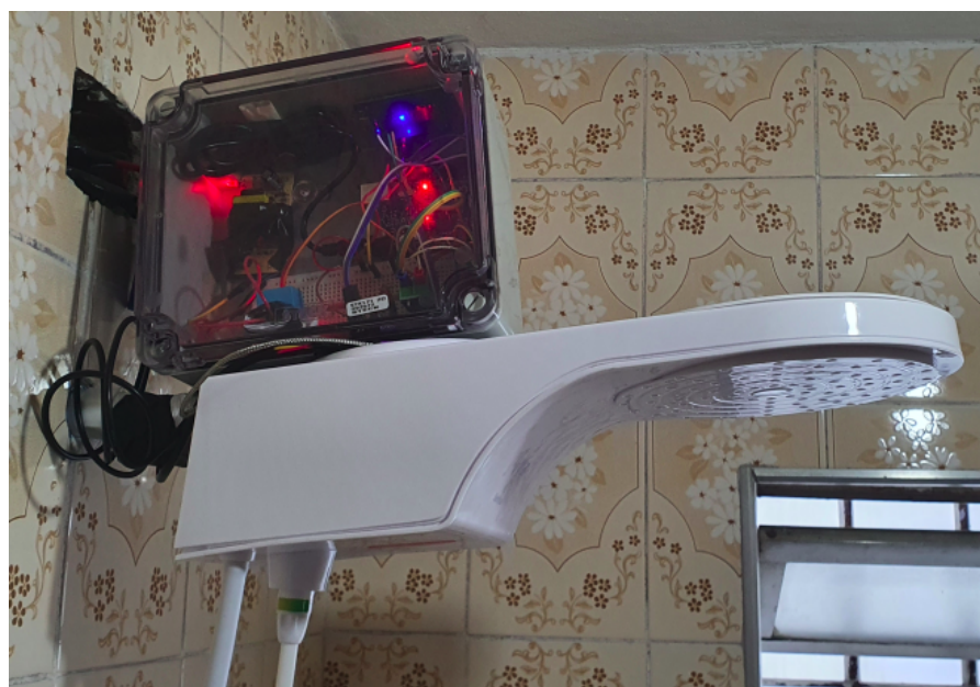
Figure 15. Installation of the shower together with the prototype.
