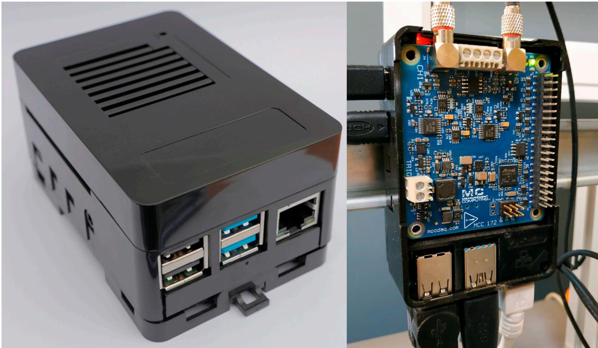
**Figure 1.** Assembled IIoT gateway.
