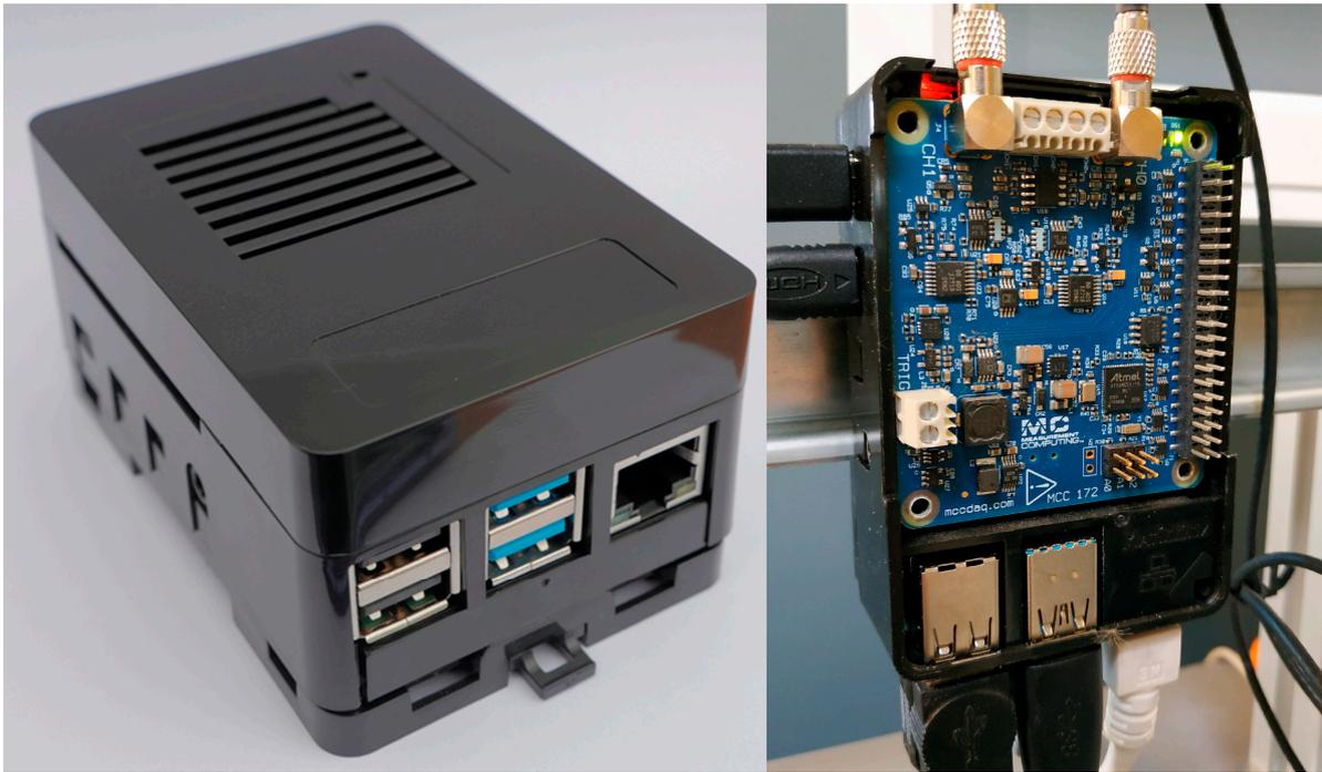
**Figure 1.** Assembled IIoT gateway.
