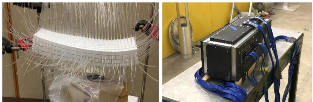
**Figure 6.** (Left) US–Japan prototype with a size of  $8 \times 8 \times 32 \text{ cm}^3$  assembled on fishing lines. (Right) US–Japan prototype in a mechanical case with attached cables.
