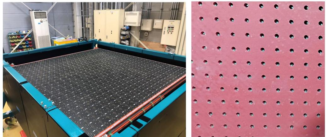
**Figure 18.** (Left) top panel of the SuperFGD with the MPPC64-PCBs attachment. (Right) WLS fibers with cutting ends before the installation of the LED calibration system.
