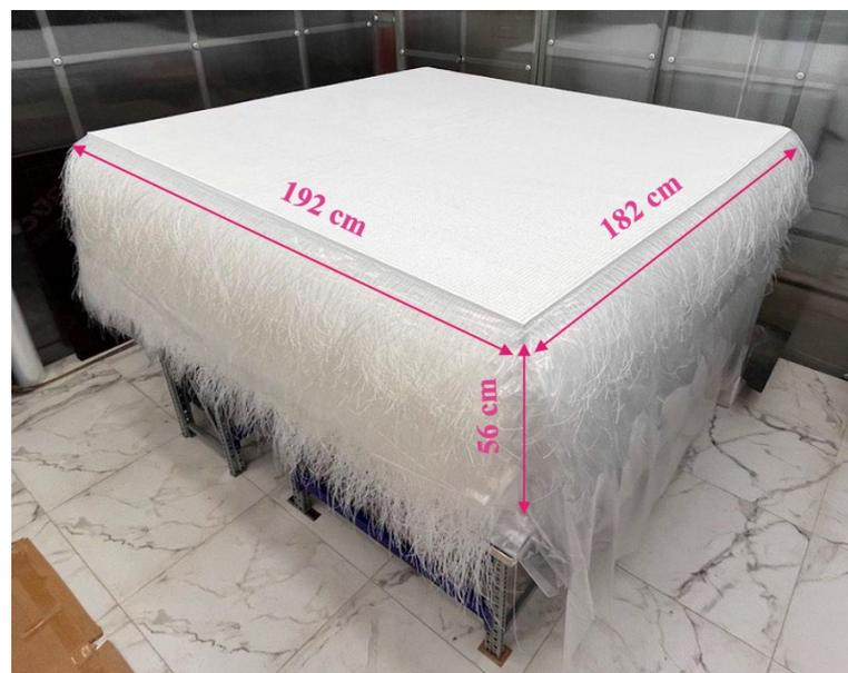
**Figure 3.** View of the SuperFGD assembled with fishing line method. The fishing lines to be replaced by wavelength shifting (WLS) fibers later.
