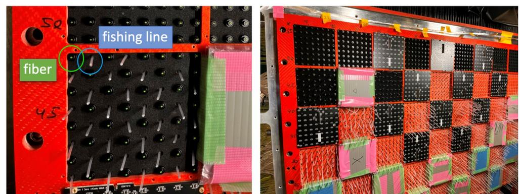
**Figure 17.** (Left) a single  $8 \times 8$  unit of through holes on the upstream panel. (Right) general view of the upstream panel during the replacement of horizontal fishing lines with the WLS fibers.
