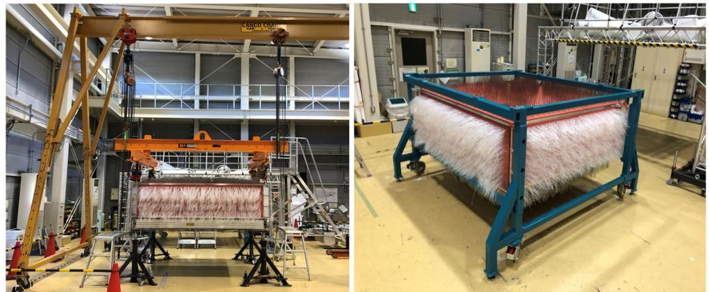
**Figure 16.** (Left) the process of the SuperFGD transportation to the mini Baby-Basket using crane equipment and the lifting device. (Right) SuperFGD inside the mini Baby-Basket frame.
