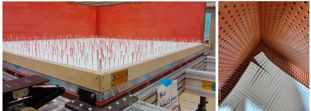
**Figure 14.** (Left) several SuperFGD layers stacked on top of each other using a stop panel and a set of steel spokes. (Right) the first SuperFGD layer on the bottom panel of the mechanical box.
