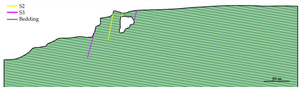
Figure 10. Geotechnical CC' cross-section; the yellow and magenta lines represent the main identified joints, while the gray lines indicate the limestone bedding.
