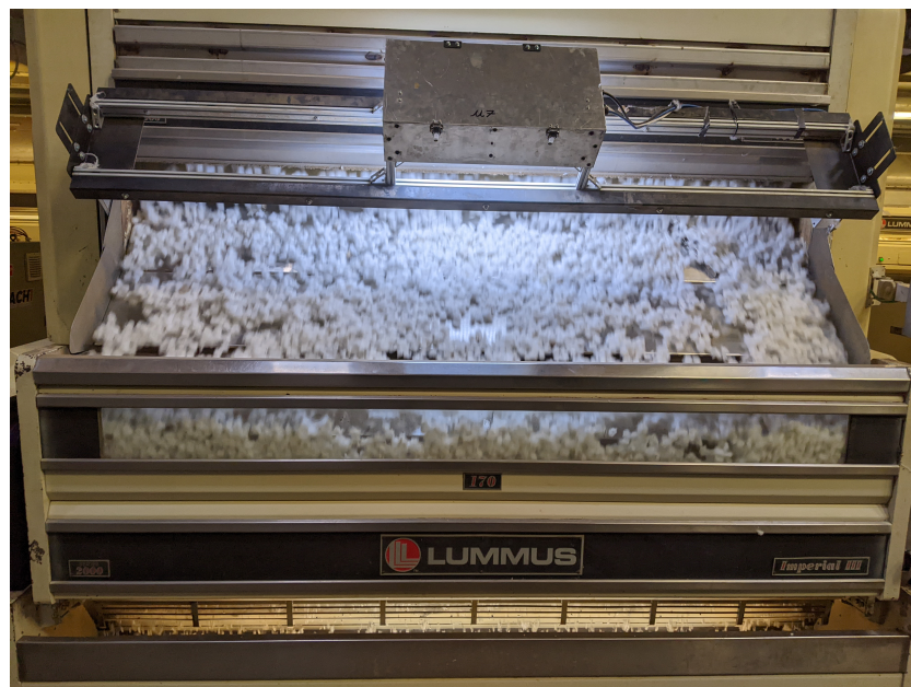
Figure 1. Optical detection system (VIPR™) deployed on a gin stand. Photograph taken at the United Cotton Growers gin in Lubbock, Texas.
