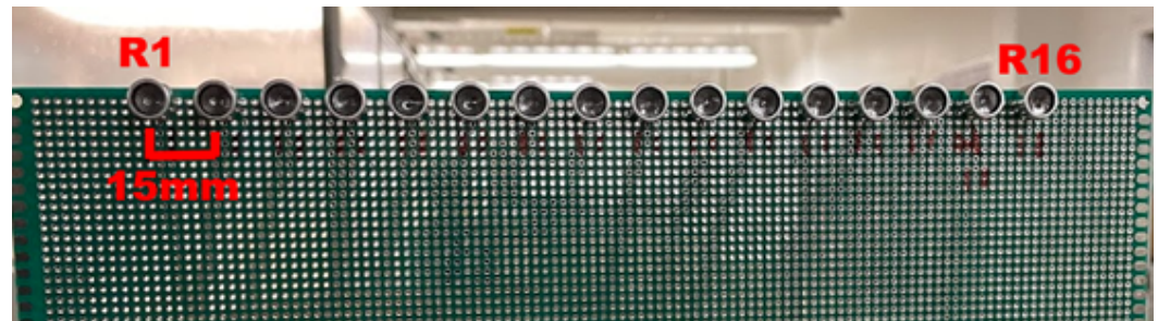
Figure 4. Linear transmission receiver layout (16 channels).
