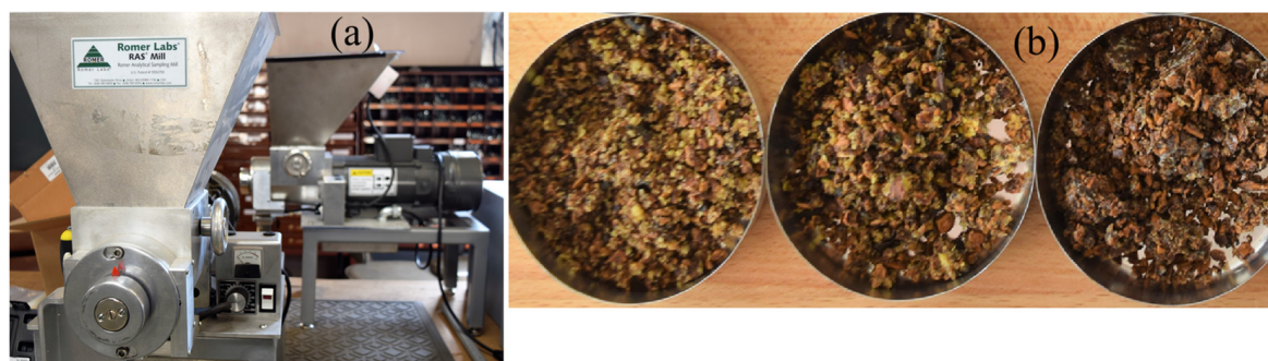
Figure 8. (a) Mill used for walnut grinding; (b) ground walnut samples.
