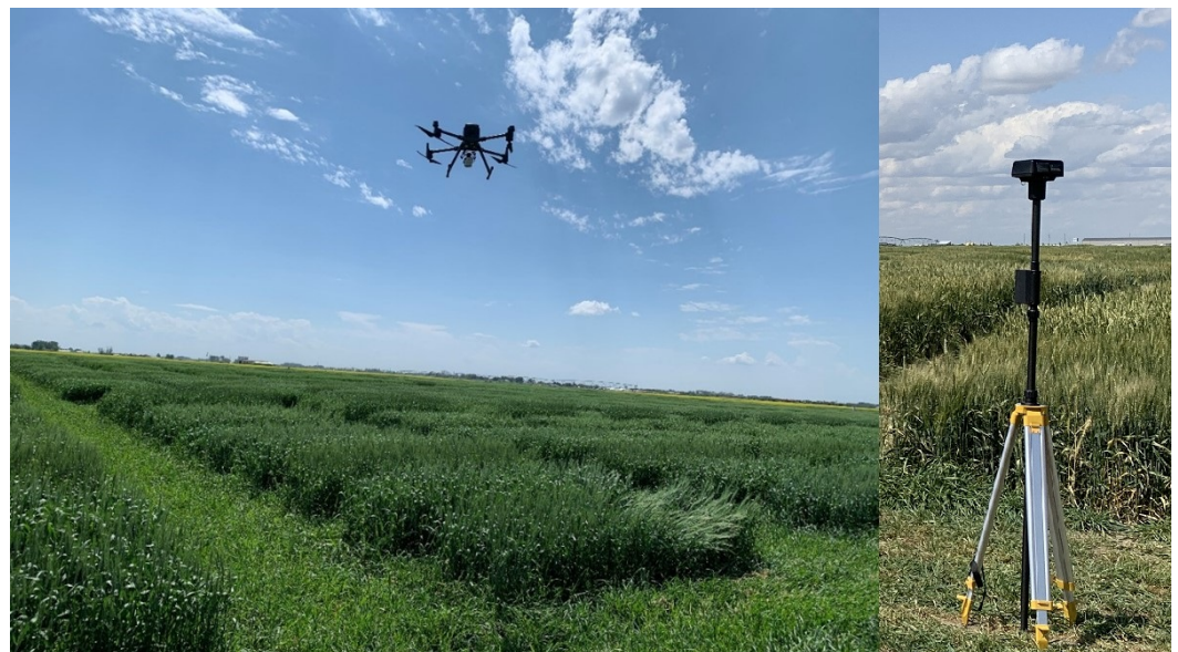
Figure 3. UAV system with the mounted multispectral camera ( left ) and a D-RTK 2 base station ( right ) for high-resolution canopy imaging over the spring wheat trial.
