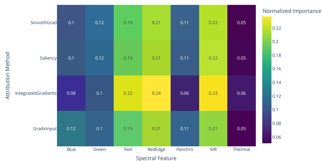
Figure 9. Feature importance of the deep learning model derived from four attribution methods (Gradient \times Input, Integrated Gradients, Saliency, and SmoothGrad) applied over 100 runs.
