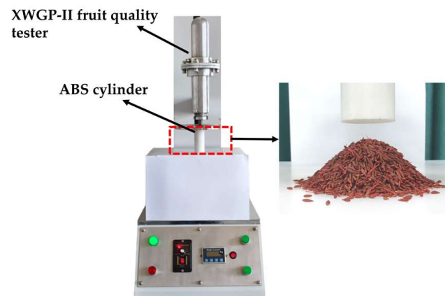
Figure 9. Physical angle of repose test for cumin seeds.
