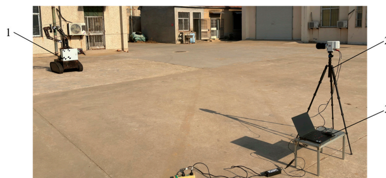
Figure 18. Experimental site for position tracking test. 1. Harvesting Device; 2. High-Speed Camera; 3. ThinkBook Mobile Computer.
