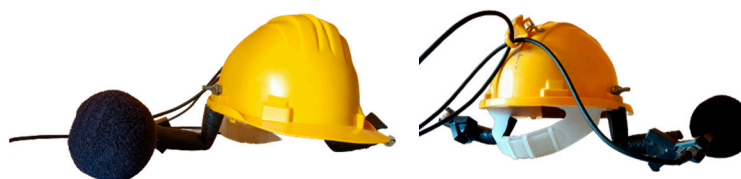
Figure 3. Patented device used to place phonometric microphone.
