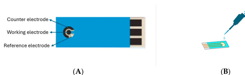
Figure 1. (A) Commercially purchased SPE with carbon WE and CE and Ag/AgCl as RE; (B) drop casting of 5 \mu\text{L} of analyte on the WE surface.
