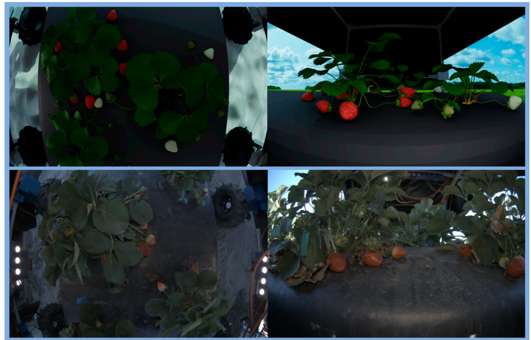
Figure 10. Comparison between images taken from a simulated camera sensor of the digital twin strawberry farm bed ( top row ) and images from a real camera taken of the field strawberry bed ( bottom row ).
