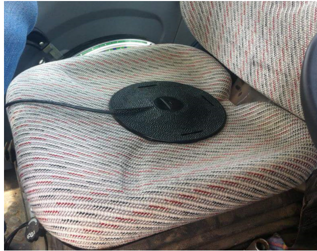
Figure 1. Sensor for measuring whole-body vibrations of an agricultural tractor operators.
