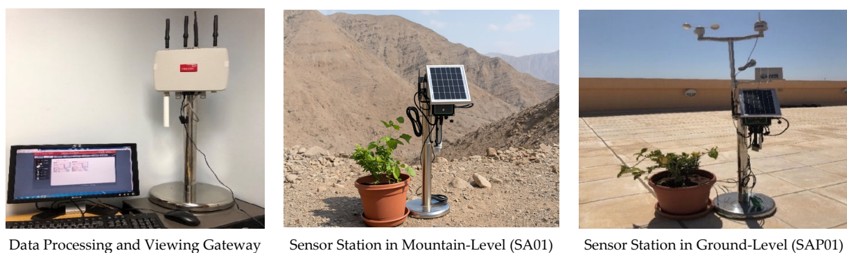
Figure 4. A schematic diagram of the experimental design and setup. Heterogeneous weather stations (SAP01 and SA01) equipped with multiple sensors collect environmental data. The data streams are transmitted to a central processing gateway.
