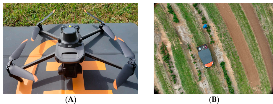
Figure 2. Unmanned aerial vehicle (UAV) and aerial imagery: (A) DJI Mavic 3 Enterprise UAV deployed during field data collection, equipped with 20 MP camera for capturing RGB images used in vegetation and flower coverage analysis; (B) Individual RGB image of blackberry plots captured at 12 m altitude.
