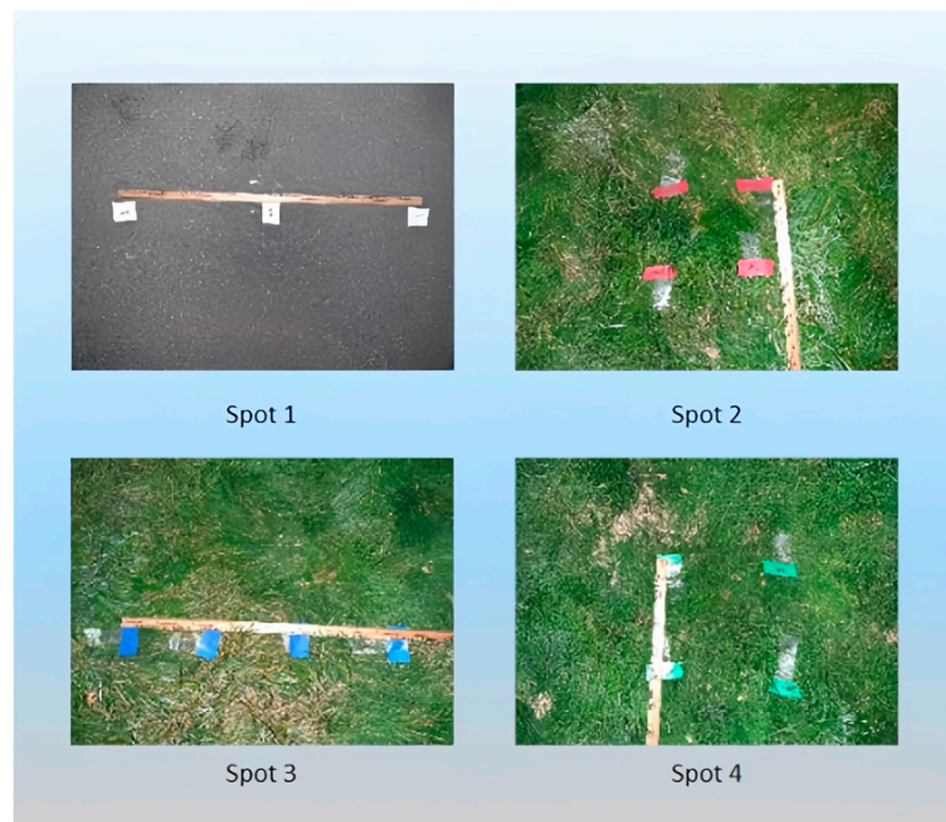
Figure 8. RTK rover's centimeter level accuracy test spots with scale to assist measurements (Spot 1: a straight line with an intermediate distance of 50 cm; Spot 2: a square with a side length of 20 cm; Spot 3: a straight line with an intermediate distance of 20 cm; Spot 4: a square with a side length of 30 cm).
