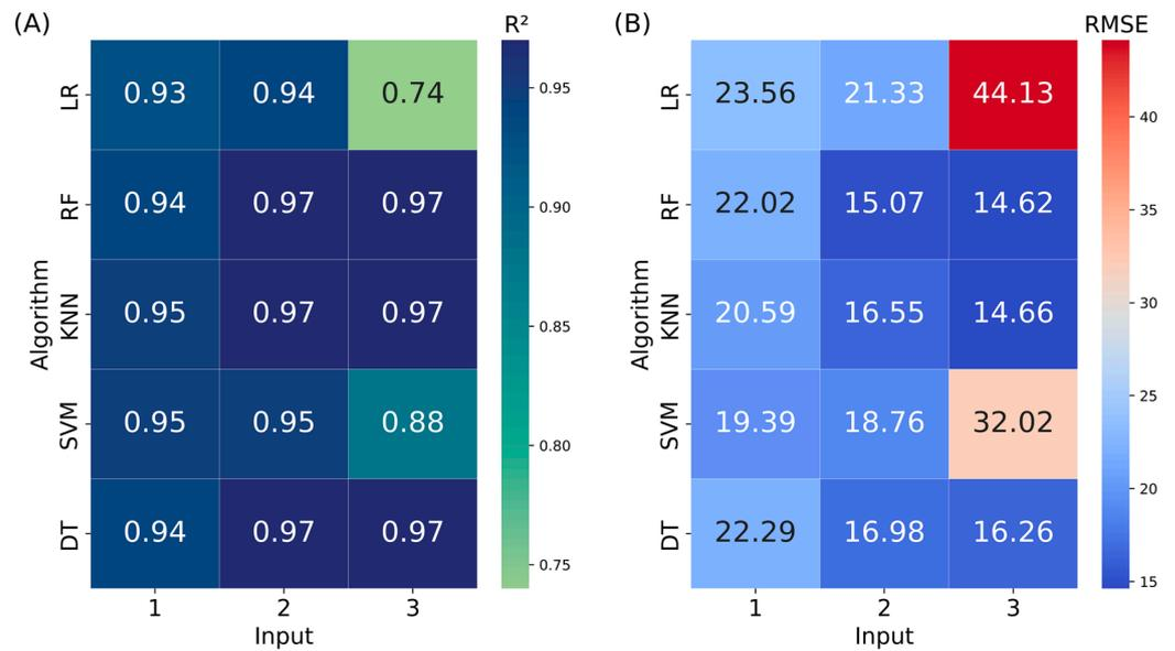
**Figure 4.** Coefficient of determination (R<sup>2</sup>) (A) and root-mean-square error (RMSE) (B) in centimeters of the ML algorithms implemented in the study.
