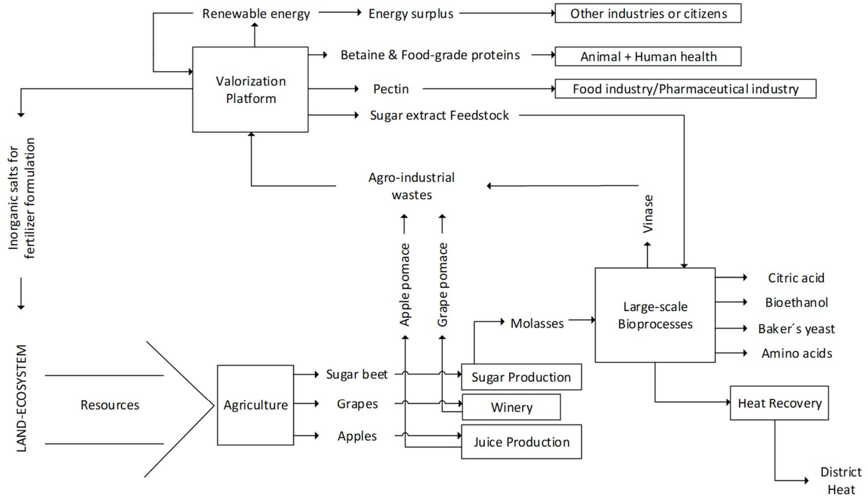
**Figure 3.** A circular flow diagram to bridge the implementation gap between agro-industrial wastes and large-scale bioprocesses. It connects agriculture and post-harvest transformation with the industrial biotechnology and other industries through the substantial valorization of vinasse, apple pomace and grape pomace into renewable energy (solid biofuels), betaine, food-grade proteins and sugar extracts as feedstock for large-scale bioproductions.
