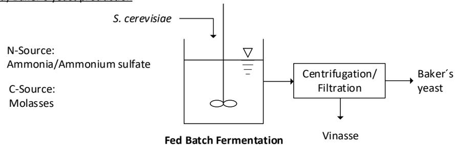
**Figure 1.** Flow diagrams for the production of bioethanol, amino acids, citric acid, and baker's yeast.
