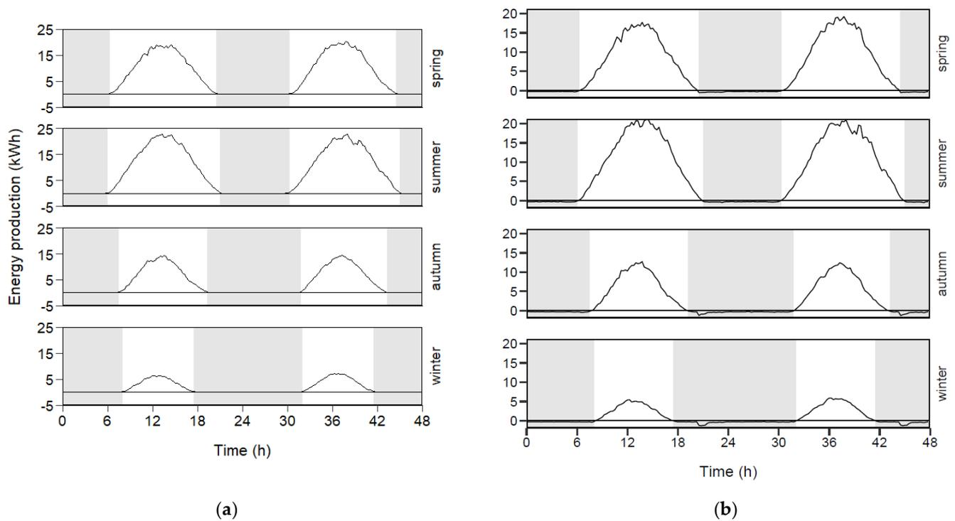
**Figure 2.** Energy production of the PV plant in 15 min resolution for a 48.00 h period (a); energy balance of the milk production system and the PV plant in a 48.00 h period (b). Periods with negative energy balance are indicated with grey areas.
