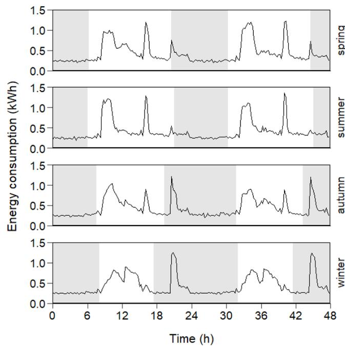
**Figure 4.** Mean energy consumption of the milking system in 15 min resolution for a 48.00 h period; periods with negative energy balance are indicated with grey areas.
