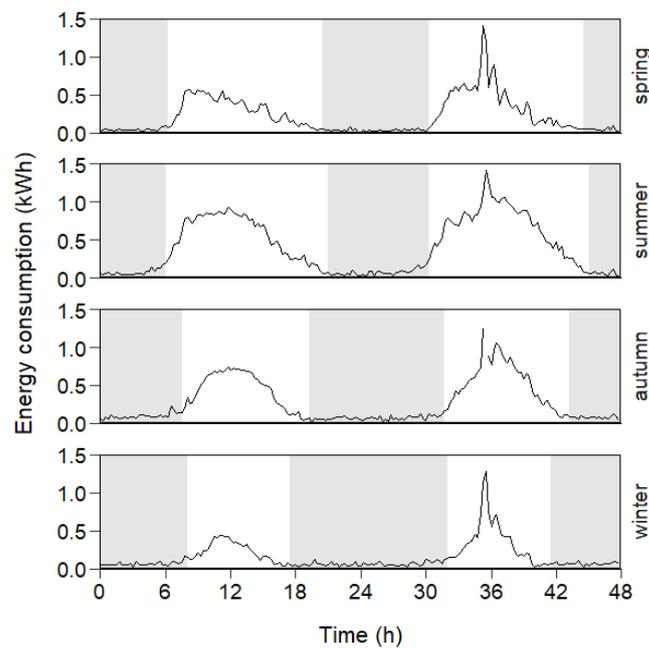
**Figure 6.** Mean energy consumption of the milk cooling system in 15 min resolution for a 48.00 h period; periods with negative energy balance are indicated with grey areas.
