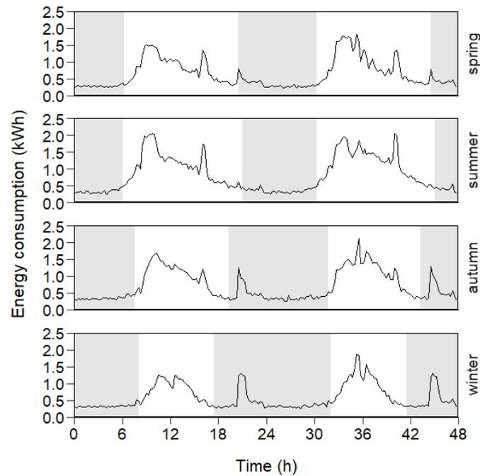
**Figure 3.** Mean energy consumption of the milk production system in 15 min resolution for a 48.00 h period; periods with negative energy balance are indicated with grey areas.
