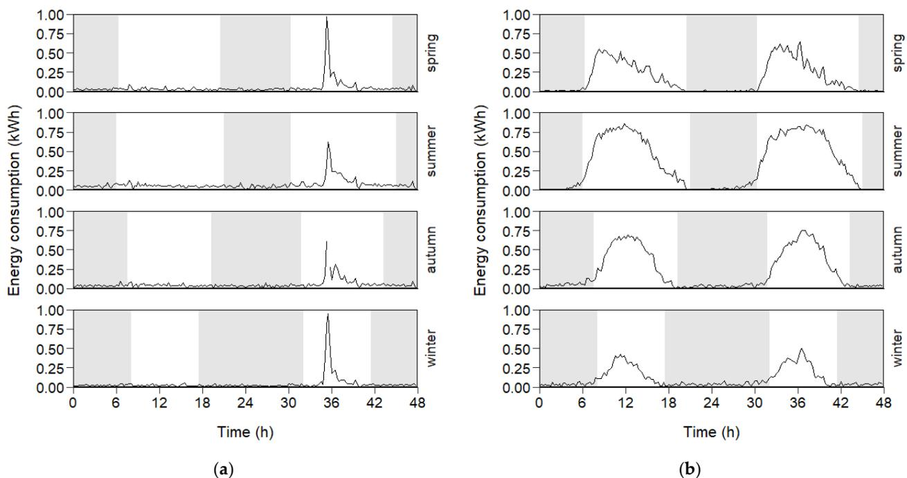
**Figure 7.** Mean energy consumption of the milk cooling tank (a) and cooling unit (b) during 48.00 h period with a resolution of 15 min; periods with negative energy balance are indicated with grey areas.
