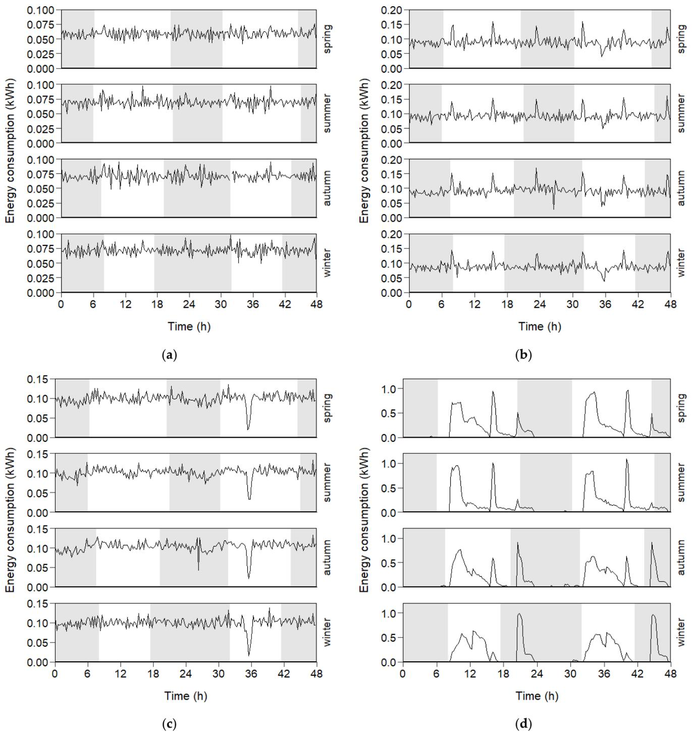
**Figure 5.** Mean energy consumption of the milking robot (a), the air compressor (b), the vacuum pump (c) and BWAC (d) during 48.00 h period with a resolution of 15 min; periods with negative energy balance are indicated with grey areas.
