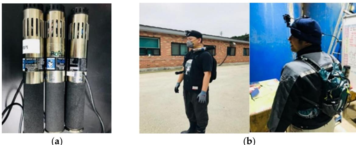
**Figure 4.** Research procedure for modeling ventilation efficiency considering regional thermal conditions. (a) NH<sub>3</sub> and H<sub>2</sub>S sensors and (b) installation of sensors at worker’s shoulder.
