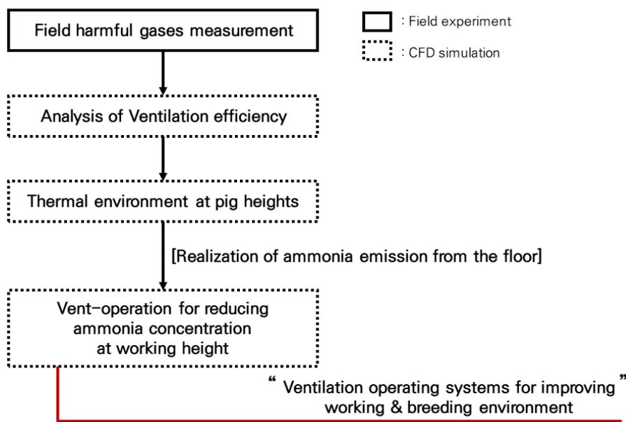
Figure 3. Research procedure for modeling ventilation efficiency considering regional thermal conditions.
