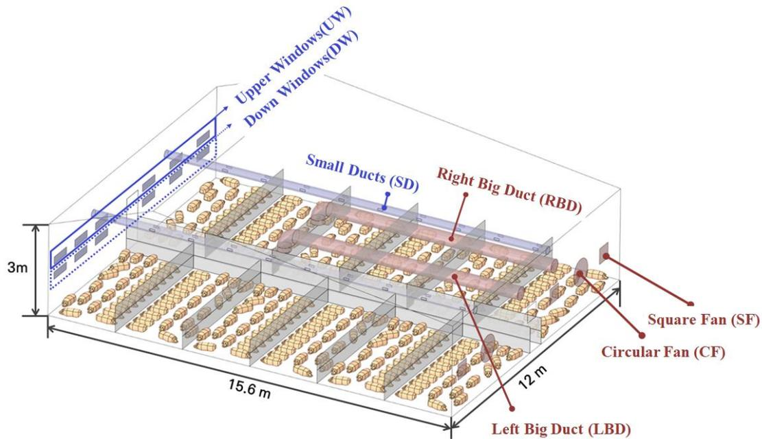
**Figure 2.** Ventilation system operated during spring season with combinations of various outlets (red) and inlets (blue).
