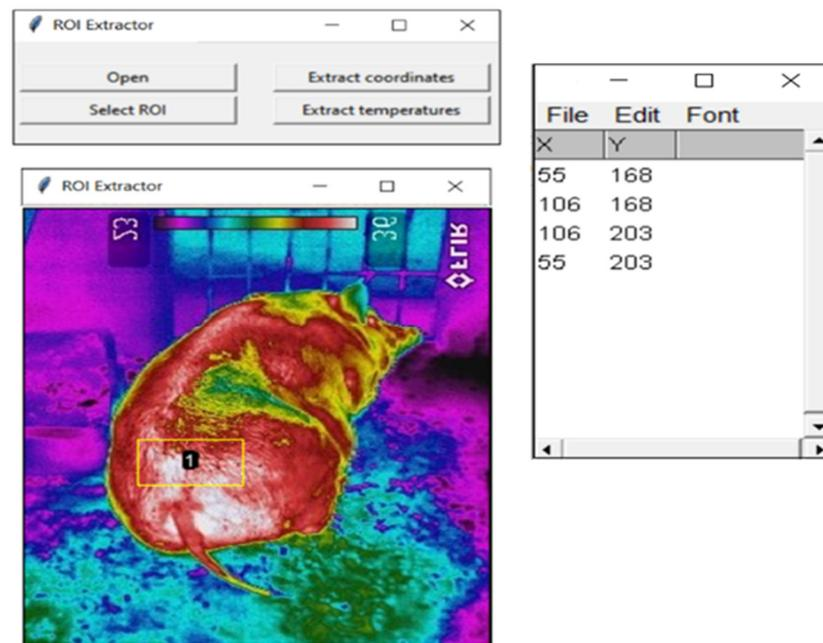
**Figure 2.** Interface developed for extracting the coordinates from the thermal image. Note: The number 1 represents a point sampled in the caudal dorsal region.
