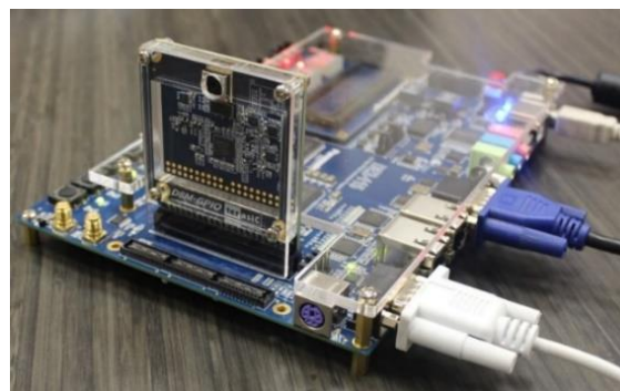
Figure 4. DE2-115 development board connected with the D8 M camera board.
