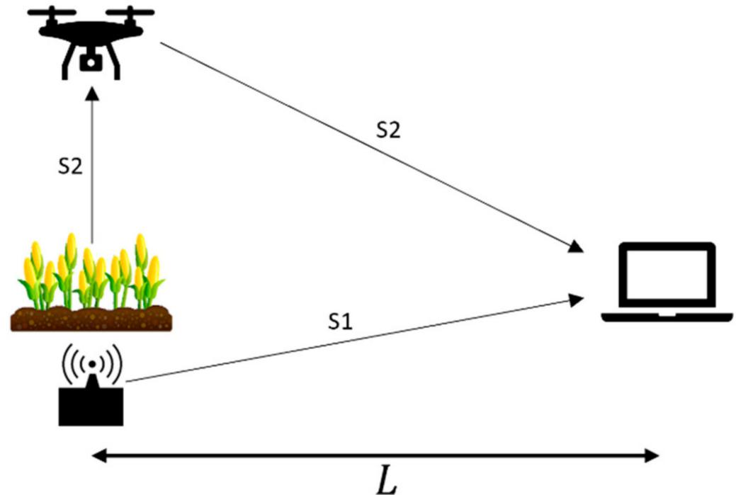
**Figure 3.** Schematic of the experimental setup used for demonstrating the extended range of the data collection system design. S1 shows the direct sensor node to ground station communication path and S2 the path with intermediate signal repetition at the drone.
