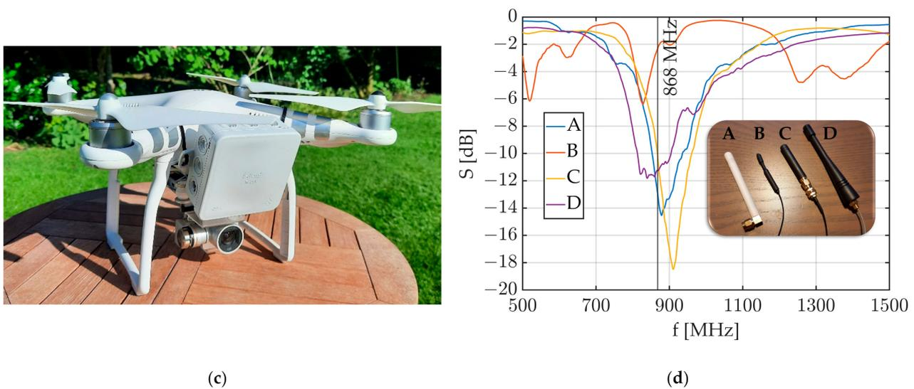
**Figure 1.** (a) Schematic of the investigated communication setup. (b) Picture of a sensor node deployed in a maize field before closing the hole with soil. (c) Picture of the drone with attached component housing. (d) Characterization of different antennas in the range around the 868 MHz LoRa frequency with the scattering parameter  $S$ .
