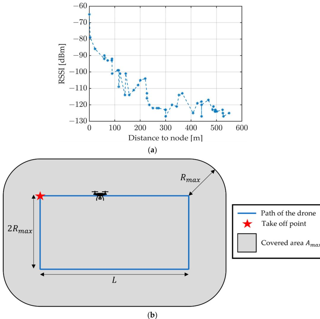
**Figure 9.** (a) Reduction in the RSSI with the increasing distance between the sensor node and drone. The sensor node depth was 30 cm. The drone had a constant flight height of 30 m. (b) Schematic of the assumed flight configuration for calculating the maximum covered area  $A_{max} = 470$  ha.
