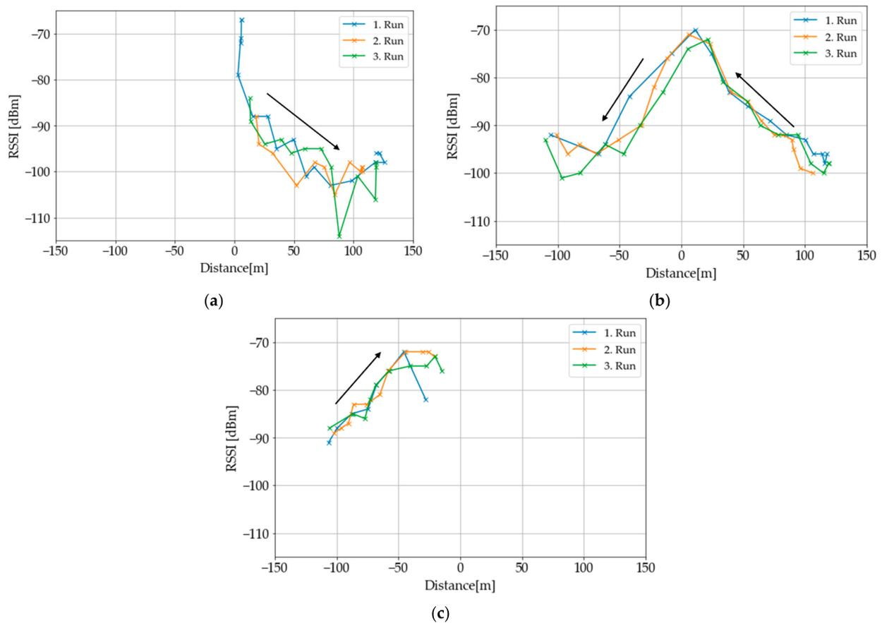
**Figure 12.** RSSI over distance diagram of the three flights, divided into the different flight phases for better clarity. The arrows show the direction of time evolution. Sensor node depth is 30 cm. Drone has a constant flight height of 25 m. (a) Phase 1. (b) Phase 2. (c) Phase 3.
