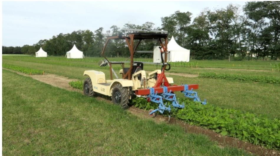
**Figure 1.** SabiAgri electrical and automatized tractor used for full-scale experiments.
