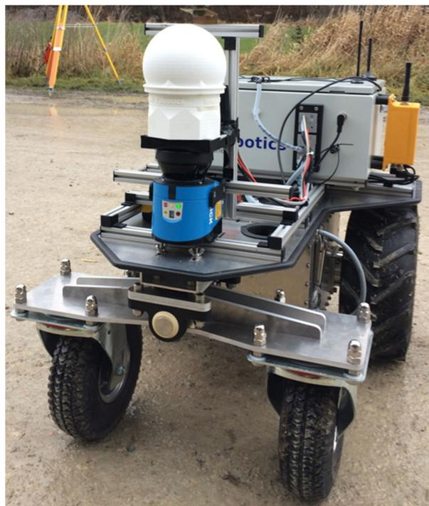
**Figure 4.** The robot vehicle with a laser scanner (blue-black) and radar scanner in the early prototype stage (white). (Own recordings).
