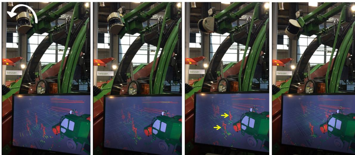
**Figure 3.** The sequence of images shows the clockwise rotation of the 2D laser scanner (white arrow) in the direction of travel and the output of the processed scanner data as a 3D point cloud on a monitor. Visitors to the fair can be seen passing by (yellow arrows). (Own recordings).
