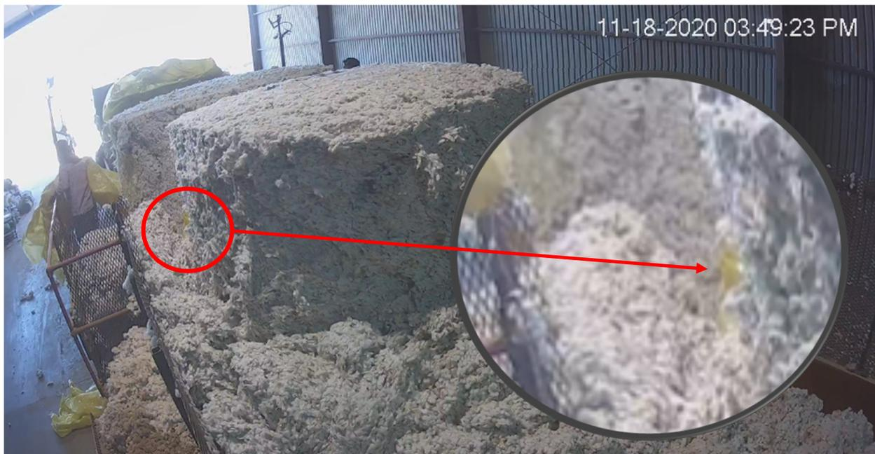
**Figure 14.** Still image from the unloading video captured for module SN 19410229688 showing a piece of yellow plastic remaining in cotton between modules (inside red circle) after the wrap was removed from the top of the module.
