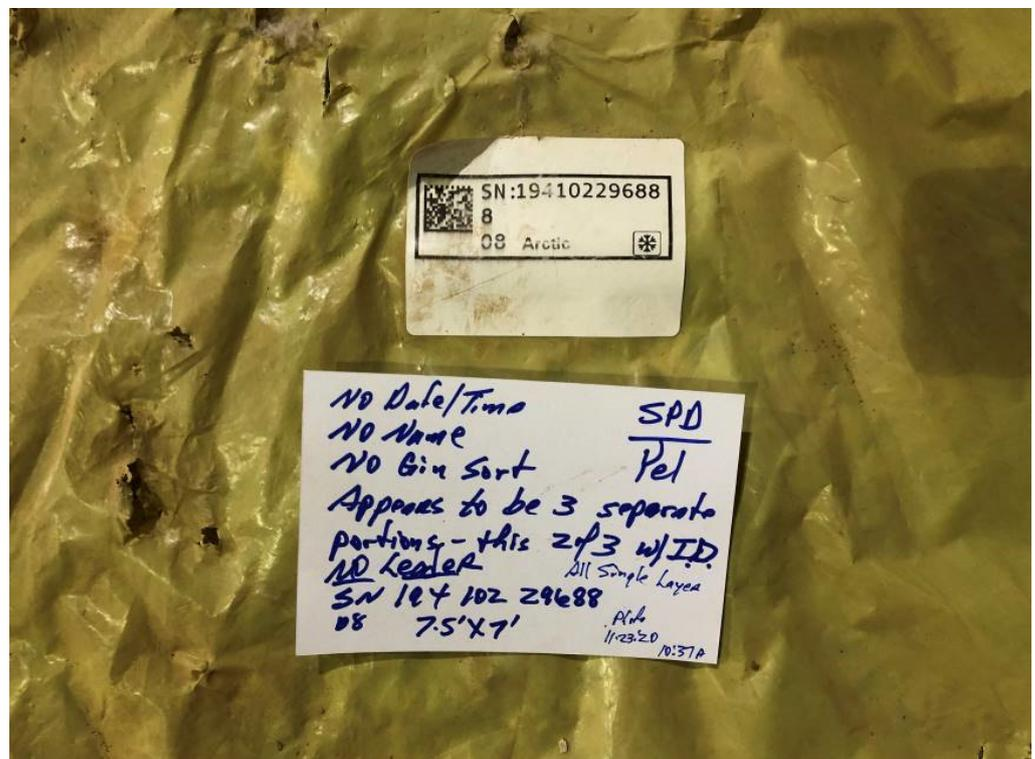
Figure 13. Image of yellow plastic removed from lowest dispersing roller (Figure 11) showing RFID tag with serial number 19410229688 that was used to identify the module from which the plastic originated.
