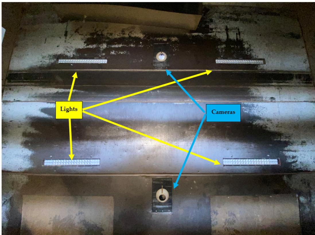
**Figure 4.** Photo of USDA Module Feeder Inspection system (MFIS) IP cameras and supplemental lights installed in the back wall of a module feeder to monitor contamination accumulation on upper and lower dispersing cylinders.
