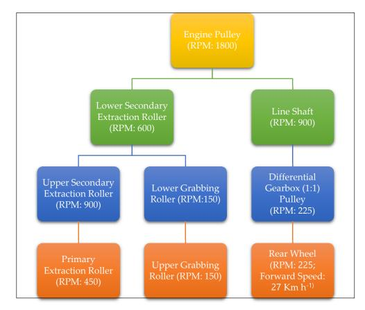
Figure 9. The power transmission system of the modified Aashkol.
