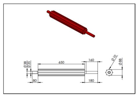
Figure 7. Schematic views of the grabbing rollers of the Aashkol.
