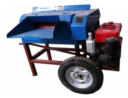
Figure 1. Pictorial view of the jute fiber extraction machine of the KP model.
