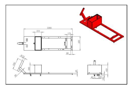
Figure 8. Schematic view of the base frame of Aashkol.
