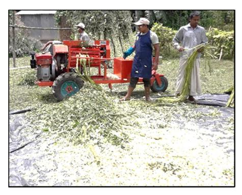
Figure 11. Jute fiber extraction by the developed Aashkol.
