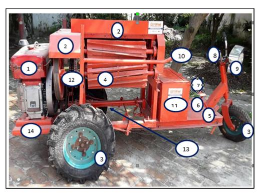
**Figure 3.** Different components of Aashkol are shown in the pictorial view from the side. 1. Engine; 2. Protection cover; 3. Wheels (two types); 4. Extraction roller; 5. Throttle lever/accelerator; 6. Brake; 7. Main clutch; 8. Handle; 9. Head light; 10. Fiber collection stand; 11. Seat cum toolbox; 12. Sprocket; 13. Differential gearbox; 14. Base frame.
