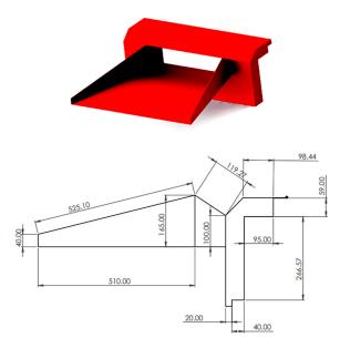
Figure 5. Isometric view of the feeding tray of the Aashkol.
