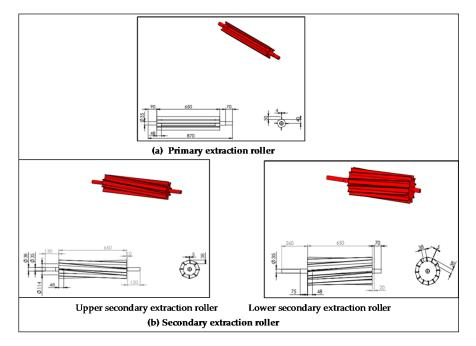
Figure 6. Schematic views of primary and secondary extraction rollers of the Aashkol.
