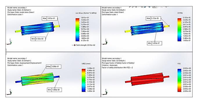
Figure 14. Stress, strain, displacement, and factor of safety of secondary extraction roller with a 200 N force considered.
