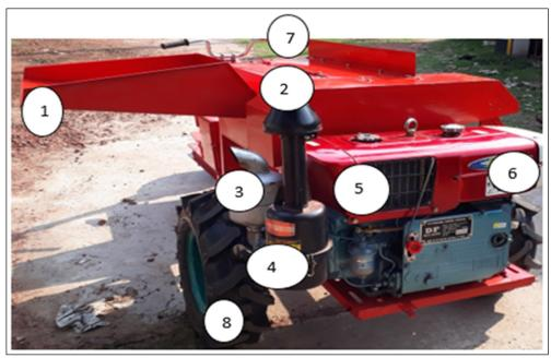
**Figure 4.** Different components of the Aashkol are shown in the pictorial view from the back. 1. Feeding tray; 2. Protection cover; 3. Silencer; 4. Air cleaner; 5. Coolant tank; 6. Fuel tank; 7. Handle, 8. Wheel.
