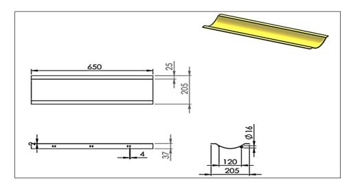
Figure 10. Schematic view of the spring-loaded tray of the Aashkol.
