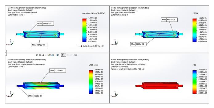
Figure 13. Stress, strain, displacement, and factor of safety of primary extraction roller with a 200 N force considered.
