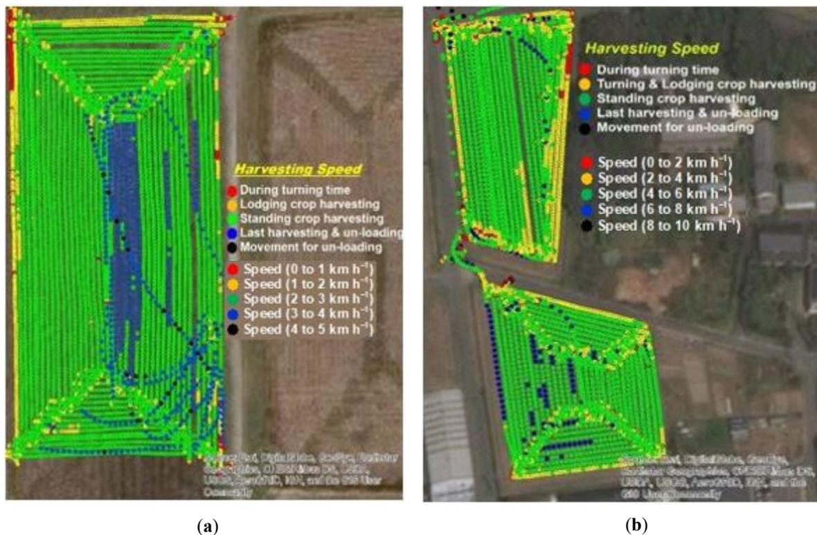
**Figure 5.** Harvester speed variations: (a) Plot 1 at Gifu University; (b) Plots 2 and 3 at Kaizu. Speed variations are presented by 5 different colors: red, yellow, green, blue, and black. The values of different speed ranges are classified from 0 to 1, 1 to 2, 2 to 3, 3 to 4, and 4 to 5  $\text{km h}^{-1}$  for the medium combine and from 0 to 2, 2 to 4, 4 to 6, 6 to 8, and 8 to 10  $\text{km h}^{-1}$  for the large combine and are shown in red, yellow, green, blue, and black, respectively.
