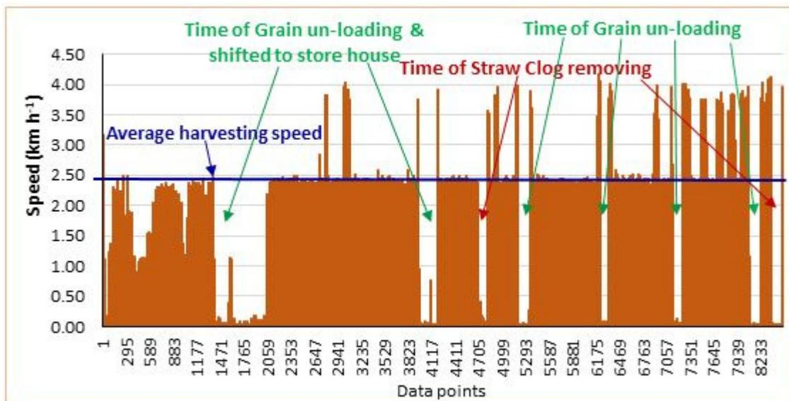
Figure 6. Different speeds and idle times during harvesting at Plot 1 by medium combine.
