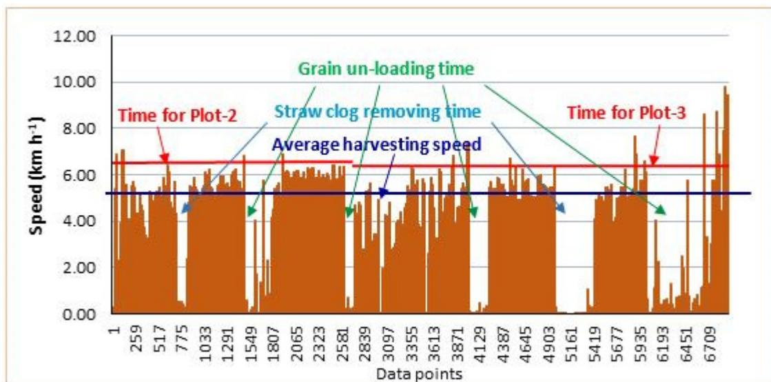
Figure 7. Different speeds and idle times during harvesting at Plots 2 and 3 by large combine.
