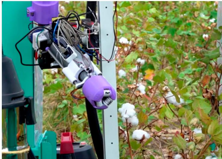
**Figure 9.** Green Robot Machinery (gRoboMac) manipulator trying to get the cotton boll (source: [www.grobomac.com](http://www.grobomac.com)).
