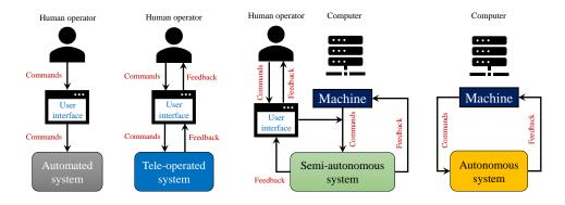
Figure 1. Automated/tele-operated, semi-autonomous, and autonomous system concepts.
