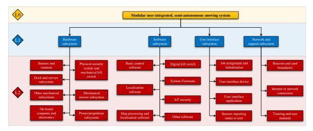
Figure 8. Proposed modular system architecture (first three levels).
