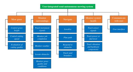
Figure 2. Example functional decomposition diagram (FDD) for a user-integrated semi-autonomous mowing system.
