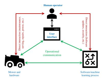
Figure 4. Semi-autonomous mowing system top-level interfaces.
