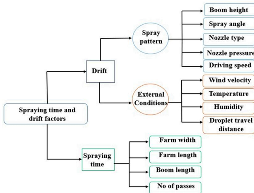
Figure 1. Drift-causing factors and spraying-speed parameters under consideration.
