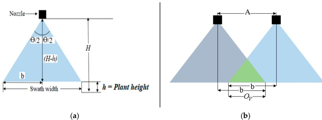
Figure 3. Swath width (a) and spray sheet overlap between consecutive nozzles (b).
