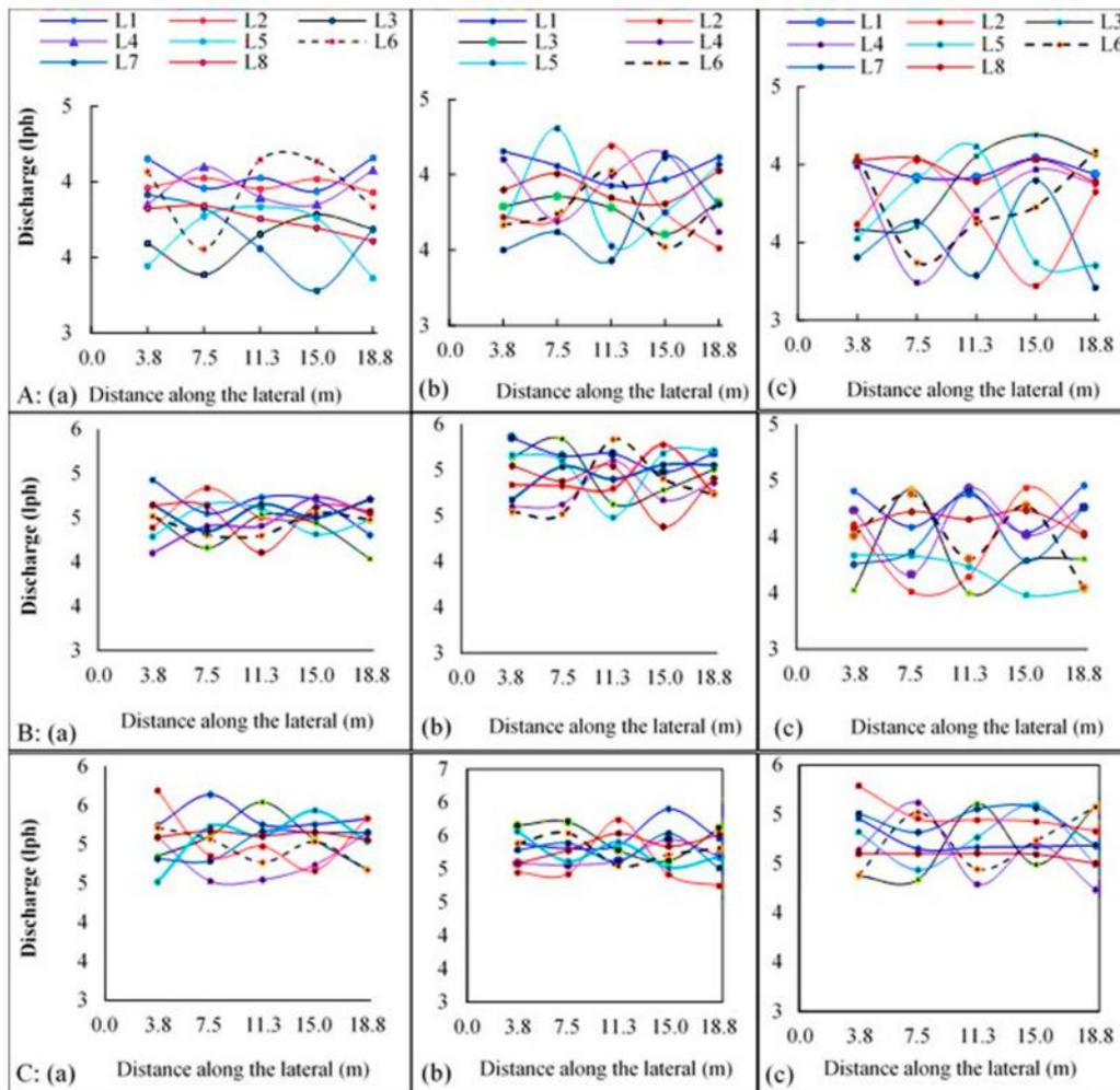
**Figure 4.** Emitter discharge rates along the lateral length at different operating pressures with various slopes, (A) 1.5 m operating pressures with (a) 0%, (b) 1%, and (c) 1.5% slope; (B) 2.0 m operating pressures with (a) 0%, (b) 1%, and (c) 1.5% slope; and (C) 2.5 m operating pressures with (a) 0%, (b) 1%, and (c) 1.5% slope.
