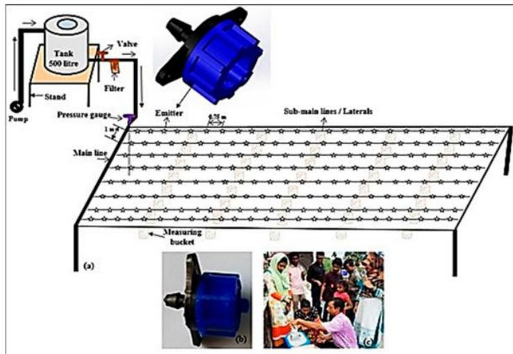
**Figure 1.** A schematic view of low pressure (gravity) drip-irrigation layout (a), new emitter (b), and measurement of each emitter discharge for characterization of hydraulic parameters (a,c).
