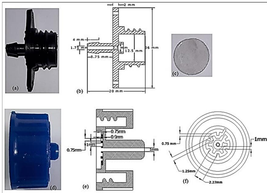
**Figure 2.** View of emitter properties and cross sectional view with leveling: (a) upper part of emitter and (b) cross section of the upper part, (c) silicon rubber washer, (d) lower part of the emitter, (e) cross section of the lower part, and (f) cross section of the labyrinth.
