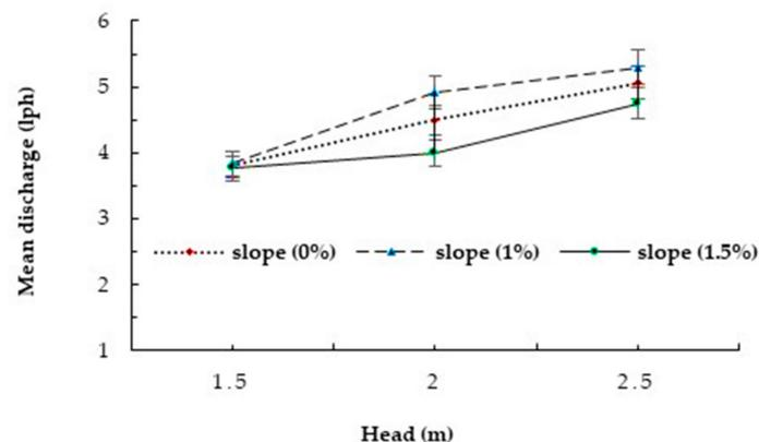
**Figure 3.** Emitter mean discharge rates for each operating pressure (head) with various slopes. Bars indicate the error percentage (5%).
