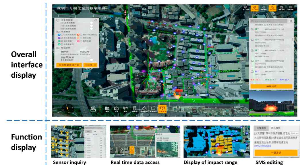
Figure 9. Fire warning and response interface display. Under “Overall interface display”: The left side is the emergency-related function panel, the middle shows scene visualization, and the right side displays specific functions.
